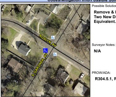
Street 1 Name Stop Condition-Street 1 Street 2 Name Stop Condition-Street 2 **S GARDNER AV** None **ROSLYN AV** StopSign Possible Solutions: Remove & Replace Curb Ramp With Two New Directional Ramps or Equivalent.
