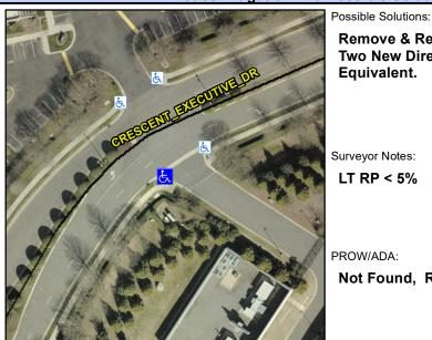
Street 1 Name None N/A Stop Condition-Street 1 Street 2 Name None Stop Condition-Street 2 CRESCENT EXECUTIVE DR Remove & Replace Curb Ramp With Two New Directional Ramps or Equivalent.
