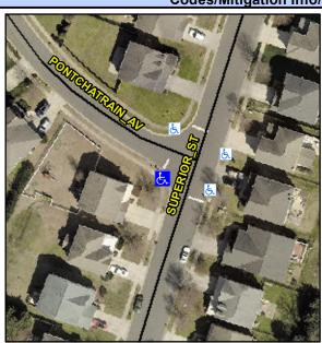
**SUPERIOR ST** Street 1 Name Stop Condition-Street 2 StopSign Street 2 Name **PONTCHATRAIN AV** Stop Condition-Street 1 StopSign Possible Solutions: **Remove & Replace Curb Ramp With** Two New Directional Ramps or Equivalent. Surveyor Notes: N/A PROW/ADA: R304.5.1, R304.5.3
