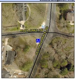
Street 1 Name Stop Condition-Street 2 Street 2 Name Stop Condition-Street 1 **OLD PROVIDENCE RD** None **RIVER OAKS LN** StopSign Possible Solutions: Remove & Replace Curb Ramp With Two New Directional Ramps or Equivalent.
