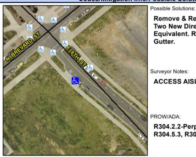
E8THST Street 1 Name Stop Condition-Street 1 None Street 2 Name N/A Stop Condition-Street 2 N/A Remove & Replace Curb Ramp With Two New Directional Ramps or Equivalent. Remove & Replace Gutter.
