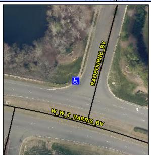
**RADBOURNE BV** Street 1 Name Stop Condition-Street 2 StopSign Street 2 Name N/A Stop Condition-Street 1 N/A Possible Solutions: Remove & Replace Entire Ramp. Surveyor Notes: N/A PROW/ADA: R304.2.2, R304.5.3, R302.7
