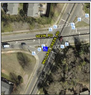
MALLARD CREEK RD Street 1 Name Stop Condition-Street 2 Signal Street 2 Name N/A Stop Condition-Street 1 N/A Possible Solutions: Remove & Replace Entire Ramp. Surveyor Notes: N/A PROW/ADA: Not Found, R304.2.2
