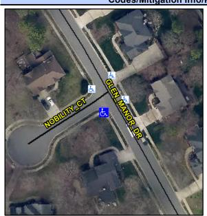
Street 1 Name Stop Condition-Street 2 Street 2 Name Stop Condition-Street 1 **GLEN MANOR DR** None **NOBILITY CT** StopSign Possible Solutions: Remove & Replace Curb Ramp With **Two New Directional Ramps or** Equivalent. Surveyor Notes: N/A PROW/ADA: Not Found, R304.5.1, R304.2.2
