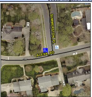
**ALEXA RD** Street 1 Name Stop Condition-Street 2 None Street 2 Name **SUMMERSTON PL** Stop Condition-Street 1 StopSign Possible Solutions: Remove & Replace Curb Ramp With **Two New Directional Ramps or** Equivalent. Surveyor Notes: N/A PROW/ADA: R304.5.1, R304.2.2, R304.5.3
