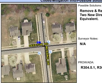
Street 1 Name Stop Condition-Street 2 Street 2 Name Stop Condition-Street 1 **DEERTON RD** None **MUNSING DR** StopSign **Remove & Replace Curb Ramp With Two New Directional Ramps or** Equivalent.
