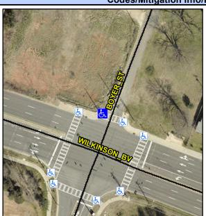
**BOYER ST** Street 1 Name Stop Condition-Street 1 Signal Street 2 Name N/A Stop Condition-Street 2 N/A Possible Solutions: Remove & Replace Entire Ramp. Surveyor Notes: RT RP <5% PROW/ADA: R304.3.2, R304.5.3
