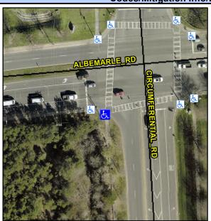
**CIRCUMFERENTIAL RD** Street 1 Name Stop Condition-Street 1 Signal Street 2 Name **ALBEMARLE RD** Stop Condition-Street 2 Signal Possible Solutions: Remove & Replace Curb Ramp With Two New Directional Ramps or Equivalent. Surveyor
