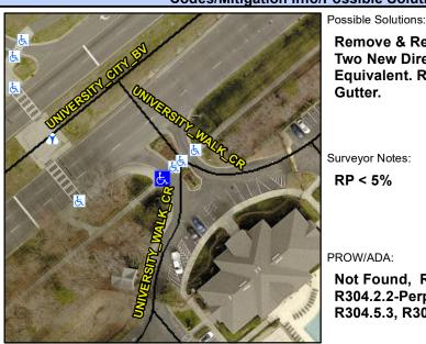
UNIVERSITY\_WALK\_CR Street 1 Name Stop Condition-Street 1 None N/A Street 2 Name Stop Condition-Street 2 N/A Remove & Replace Curb Ramp With Two New Directional Ramps or Equivalent. Remove & Replace Gutter.
