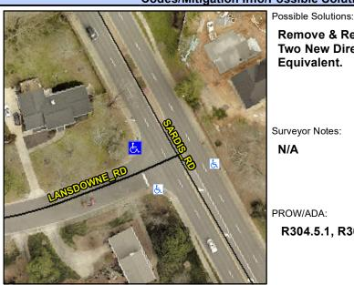
LANSDOWNE R Street 1 Name Stop Condition-Street 2 StopSig **SARDIS R** Street 2 Name Stop Condition-Street 1 Non Remove & Replace Curb Ramp With Two New Directional Ramps or Equivalent.
