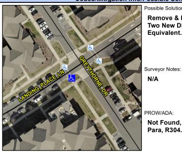
**LANDING PLACE LN** Street 1 Name Stop Condition-Street 1 None Street 2 Name N/A Stop Condition-Street 2 N/A Possible Solutions: Remove & Replace Curb Ramp With **Two New Directional Ramps or** Equivalent.
