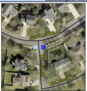
Street 1 Name Stop Condition-Street 2 Street 2 Name Stop Condition-Street 1 **SELWYN FARMS LN** None MILL RUN DR StopSign Possible Solutions: Remove & Replace Curb Ramp With **Two New Directional Ramps or** Equivalent. Surveyor Notes: N/A PROW/ADA: R304.5.1, R304.5.3
