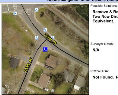
**DUNN AV** Street 1 Name Stop Condition-Street 2 Street 2 Name **GENE AV** Stop Condition-Street 1 StopSign Remove & Replace Curb Ramp With Two New Directional Ramps of Equivalent.
