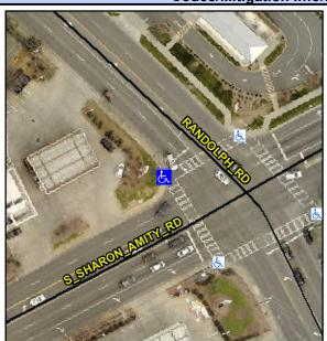
Street 1 Name N SHARON AMITY RD Stop Condition-Street 2 Signal Street 2 Name **RANDOLPH RD** Stop Condition-Street 1 Signal Possible Solutions: Remove & Replace Curb Ramp With **Two New Directional Ramps or** Equivalent. Surveyor Notes: N/A PROW/ADA: Not Found, R304.2.2
