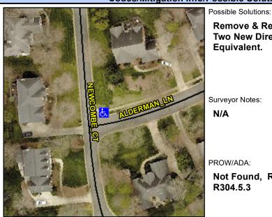
Street 1 Name Stop Condition-Street 2 Street 2 Name Stop Condition-Street 1 **NEWCOMBE CT** None **ALDERMAN LN** StopSign **Remove & Replace Curb Ramp With Two New Directional Ramps or** Equivalent.
