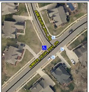
Street 1 Name Stop Condition-Street 2 Street 2 Name Stop Condition-Street 1 AMBER LEIGH WAY DR None **AMESBURY HILL DR** StopSign Possible Solutions: Remove & Replace Curb Ramp With **Two New Directional Ramps or** Equivalent. Surveyor Notes: N/A PROW/ADA: R304.5.1, R304.2.2, R304.5.3
