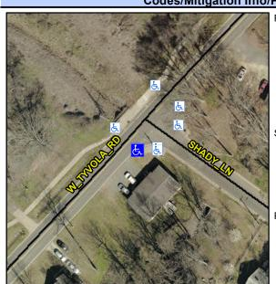
Street 1 Name None Stop Condition-Street 1 W TYVOLA RS N/A Street 2 Name Stop Condition-Street 2 N/A Possible Solutions: Remove & Replace Entire Ramp. Surveyor Notes: LT RP < 5% PROW/ADA: R304.5.1, R304.5.3, R304.3.2
