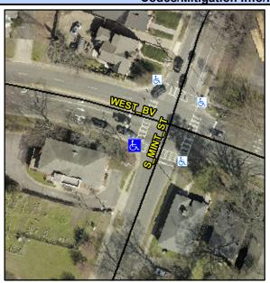
S MINT ST Street 1 Name Stop Condition-Street 2 Signal Street 2 Name **WEST BV** Stop Condition-Street 1 Signal Possible Solutions: Remove & Replace Curb Ramp With Two New Directional Ramps or Equivalent. Surveyor Notes: N/A PROW/ADA: Not Found, R304.5.1, R304.2.2
