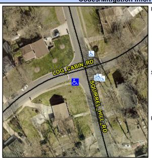
Street 1 Name None Stop Condition-Street 1 SQUIRREL HILL RD N/A Street 2 Name Stop Condition-Street 2 N/A Possible Solutions: Remove & Replace Entire Ramp. Surveyor Notes: **GTR GAP 6.0, LT RP < 5%** PROW/ADA: Not Found, R304.5.1, R304.2.2, R304.5.3, R304.3.2
