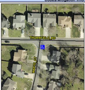
Street 1 Name Stop Condition-Street 2 Street 2 Name Stop Condition-Street 1 THORNEFIELD RD None **WAPITI CT** StopSign Possible Solutions: Remove & Replace Curb Ramp With Two New Directional Ramps or Equivalent. Surveyor Notes: N/A PROW/ADA: Not Found, R304.2.2, R304.5.3
