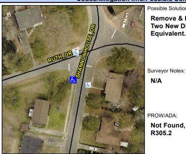
**SHANNONHOUSE DR** Street 1 Name Stop Condition-Street 1 StopSign Street 2 Name **RUTH DR** Stop Condition-Street 2 StopSign Possible Solutions: **Remove & Replace Curb Ramp With** Two New Directional Ramps or Equivalent.
