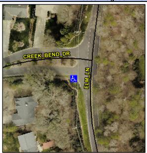
**ELM LN** Street 1 Name Stop Condition-Street 2 None **CREEK BEND DR** Street 2 Name Stop Condition-Street 1 StopSign Possible Solutions: Compliance Description N/A Remove & Replace Curb Ramp With Two New Directional Ramps or Yes Equivalent. Surveyor Notes: N/A PROW/ADA: Not Found, R304.5.3
