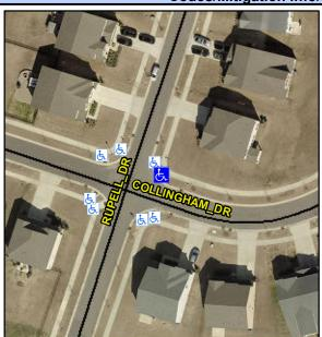
Street 1 Name **COLLINGHAM DR** Stop Condition-Street 1 None Street 2 Name N/A Stop Condition-Street 2 N/A Possible Solutions: Remove & Replace Curb Ramp With Two New Directional Ramps or Equivalent. Surveyor Notes: N/A PROW/ADA: R304.5.1
