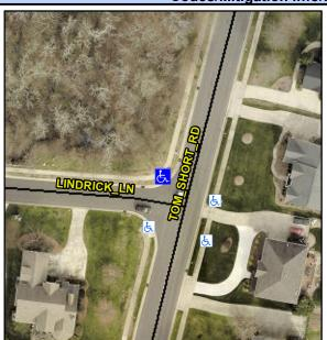
Street 1 Name StopSign Stop Condition-Street 1 LINDRICK LN Street 2 Name Stop Condition-Street 2 TOM SHORT RD Possible Solutions: Remove & Replace Curb Ramp With Two New Directional Ramps or Equivalent. Surveyor Notes: LT RP < 5% PROW/ADA: R304.5.1, R304.2.2, R304.5.3
