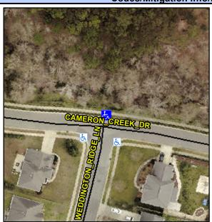
**CAMERON CREEK DR** Street 1 Name Stop Condition-Street 2 None Street 2 Name N/A Stop Condition-Street 1 N/A Possible Solutions: Remove & Replace Entire Ramp. Remove & Replace Gutter. Surveyor Notes: N/A PROW/ADA: R304.2.2-Perp, R304.3.2-Para, R304.5.3, R305, R304.5.4
