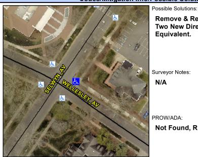
Street 1 Name Stop Condition-Street 2 Street 2 Name Stop Condition-Street 1 Remove & Replace Curb Ramp With Two New Directional Ramps or Equivalent.
