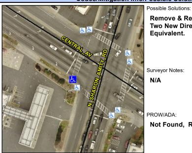
**CENTRAL AV** Street 1 Name Stop Condition-Street 1 Signal Street 2 Name N/A Stop Condition-Street 2 N/A **Remove & Replace Curb Ramp With** Two New Directional Ramps or Equivalent.
