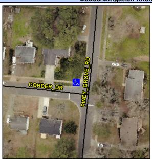
**CORDER DR** Street 1 Name Stop Condition-Street 2 StopSign **PINEY GROVE RD** Street 2 Name Stop Condition-Street 1 StopSign Possible Solutions: Compliance Description N/A Remove & Replace Curb Ramp With Two New Directional Ramps or Yes Equivalent. Surveyor Notes: N/A PROW/ADA: Not Found, R304.2.2
