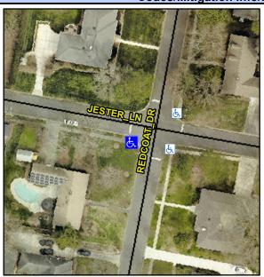
Street 1 Name Stop Condition-Street 2 Street 2 Name Stop Condition-Street 1 REDCOAT DR StopSign **JESTER LN** StopSign Possible Solutions: Remove & Replace Curb Ramp With Two New Directional Ramps or Equivalent. Surveyor Notes: N/A
