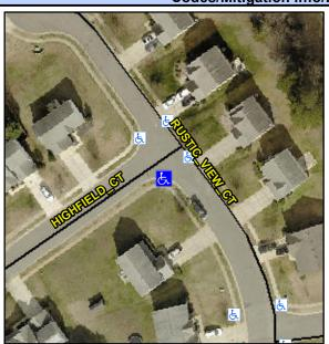
Street 1 Name Stop Condition-Street 2 Street 2 Name Stop Condition-Street 1 **RUSTIC VIEW CT** None **HIGHFIELD CT** StopSign Possible Solutions: Remove & Replace Curb Ramp With **Two New Directional Ramps or** Equivalent. Surveyor Notes: N/A PROW/ADA: Not Found, R304.5.3
