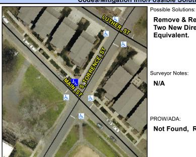
MAIN ST Street 1 Name Stop Condition-Street 2 StopSign Street 2 Name **S TORRENCE ST** Stop Condition-Street 1 StopSign Remove & Replace Curb Ramp With Two New Directional Ramps or Fauivalent
