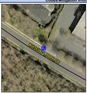
Street 1 Name WHITEHALL PARK DR Stop Condition-Street 2 None **ENTRANCE** Street 2 Name Stop Condition-Street 1 None Possible Solutions: Remove & Replace Curb Ramp With Two New Directional Ramps or Equivalent. Surveyor Notes: N/A PROW/ADA: Not Found, R304.2.2, R304.5.3
