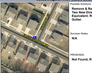
Street 1 Name Stop Condition-Street 2 Street 2 Name Stop Condition-Street 1 **EASTFIELD PARK DR** None **DUNSLOW CT** StopSign Remove & Replace Curb Ramp With Two New Directional Ramps or Equivalent. Remove & Replace Gutter.
