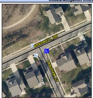
Street 1 Name Stop Condition-Street 2 Street 2 Name Stop Condition-Street 1 **BRADWELL DR** None **LANGHAM CT** StopSign Possible Solutions: Remove & Replace Curb Ramp With **Two New Directional Ramps or** Equivalent. Surveyor Notes: N/A PROW/ADA: Not Found, R304.5.1, R304.2.2
