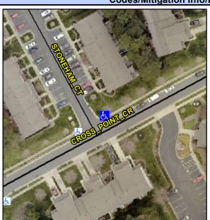
Stop Condition-Street 2 Street 2 Name Stop Condition-Street 1 STONEHAM CT StopSign Possible Solutions: Remove & Replace Curb Ramp With Two New Directional Ramps or Equivalent.
