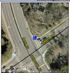
JOHNSTON RD Street 1 Name Stop Condition-Street 2 Signal Street 2 Name PARK RD Stop Condition-Street 1 Signal Possible Solutions: Remove & Replace Curb Ramp With Two New Directional Ramps or Equivalent. Surveyor Notes: N/A PROW/ADA: Not Found, R304.2.2
