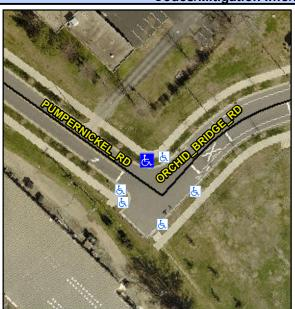
Street 1 Name **PUMPERNICKLE RD** Stop Condition-Street 2 StopSign Street 2 Name N/A Stop Condition-Street 1 N/A Possible Solutions: Remove & Replace Entire Ramp. Surveyor Notes: N/A PROW/ADA: R304.2.2, R304.5.3
