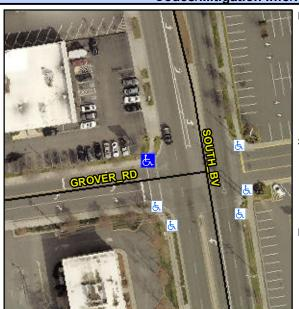
**GROVER RD** Street 1 Name Stop Condition-Street 2 StopSign Street 2 Name **SOUTH BV** Stop Condition-Street 1 None Possible Solutions: Remove & Replace Curb Ramp With **Two New Directional Ramps or** Equivalent. Surveyor Notes: N/A PROW/ADA: Not Found, R304.5.1, R304.2.2, R304.5.3
