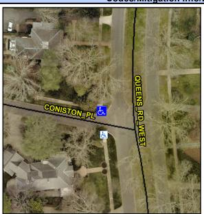
**CONISTON PL** Street 1 Name Stop Condition-Street 1 StopSign Street 2 Name N/A Stop Condition-Street 2 N/A Possible Solutions: Remove & Replace Entire Ramp. Surveyor Notes: **NO CURB LINE, MEDIAN ACROSS QUEENS RD WEST** PROW/ADA: R304.5.3
