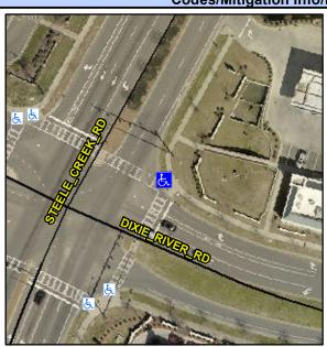
**DIXIE RIVER RD** Street 1 Name Stop Condition-Street 2 Signal Street 2 Name STEELE CREEK RD Stop Condition-Street 1 Signal Possible Solutions: Remove & Replace Curb Ramp With **Two New Directional Ramps or** Equivalent. Surveyor Notes: N/A PROW/ADA: R304.5.1
