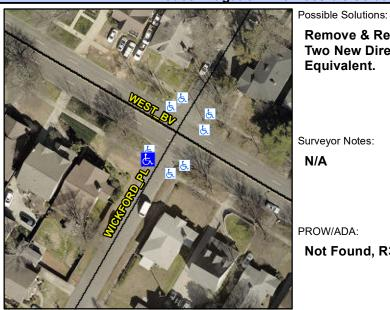
Street 1 Name **WICKFORD PL** Stop Condition-Street 1 StopSign Street 2 Name N/A Stop Condition-Street 2 N/A Remove & Replace Curb Ramp With Two New Directional Ramps or Equivalent.
