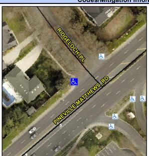
Street 1 Name Stop Condition-Street 2 Street 2 Name Stop Condition-Street 1 PINEVILLE-MATTHEWS RD None RIDGELOCH PL StopSign Possible Solutions: Remove & Replace Curb Ramp With **Two New Directional Ramps or** Equivalent. Surveyor Notes: N/A PROW/ADA: Not Found, R304.2.2, R304.5.3
