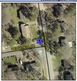
Street 1 Name Stop Condition-Street 2 Street 2 Name Stop Condition-Street 1 **WEDGEFIELD DR** StopSign **KENHILL DR** None Possible Solutions: Remove & Replace Curb Ramp With **Two New Directional Ramps or** Equivalent. Surveyor Notes: N/A PROW/ADA: Not Found, R304.5.1
