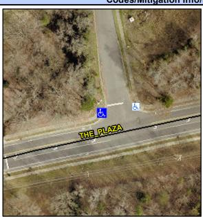
THE PLAZA Street 1 Name Stop Condition-Street 2 None Street 2 Name **ENTRANCE** Stop Condition-Street 1 StopSign Possible Solutions: Remove & Replace Curb Ramp With Two New Directional Ramps or Equivalent. Surveyor Notes: N/A PROW/ADA: Not Found, R304.5.3
