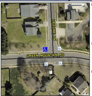
Street 1 Name **GREEN MOUNTAIN RD** Stop Condition-Street 1 None LIFELINE LN Street 2 Name Stop Condition-Street 2 StopSign Possible Solutions: Remove & Replace Curb Ramp With Two New Directional Ramps or Equivalent. Surveyor Notes: N/A PROW/ADA: R304.5.1, R304.5.3
