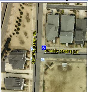
**COTTON STAND RD** Street 1 Name Stop Condition-Street 2 Street 2 Name **GRASSY CROPS RD** Stop Condition-Street 1 StopSign Possible Solutions: Remove & Replace Curb Ramp With Two New Directional Ramps or Equivalent. Surveyor Notes: N/A PROW/ADA: Not Found, R304.5.3
